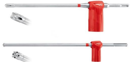
"These Hilti TE-CD hollow drill bits have been used on various CRL sites and 'do what they say they will do' - reduce the production of air-borne dust, utilising the purpose designed sleeve on the shank, attached to a class M vacuum.
